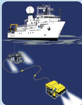
NOAA Ship Okeanos Explorer with camera sled, Seirios , deployed and below that, IFE's Little Hercules —a science-class ROV. Credit: Randy Canfield and NOAA.
