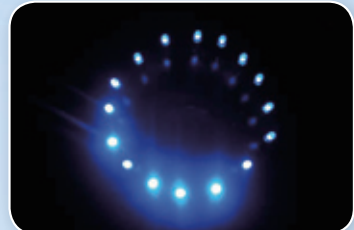
Electronic jellyfish lure of blue light emitting diodes, used to attract and communicate with deep-sea creatures. Credit: Edie Widder, Harbor Branch Oceanographic Institution.
