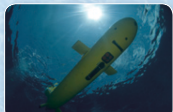
Sensors and systems on the AUV Eagle Ray produce data for a wide range of products, including maps of the seafloor to more than 7,000 feet deep. Credit: Greg McFall, NOAA.
