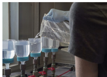
The vacuum filtration unit used to filter eDNA from sea water samples collected by ROV SuBastian. Image courtesy of SOI/Monika Naranjo Gonzalez.
