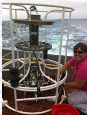
A conductivity/temperature/depth (CTD) sensor package. Image courtesy of NOAA Okeanos Explorer Program. http://oceanexplorer.noaa.gov/okeanos/explorations/ex1103/logs/july16/media/ctd.html
