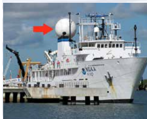
Telepresence: real-time, broadband video and audio communications made possible by the Okeanos Explorer's powerful satellite antenna (red arrow). Image courtesy of NOAA Okeanos Explorer Program, INDEX-SATAL 2010. http://oceanexplorer.noaa.gov/okeanos/explorations/10index/logs/july09/media/okeanos_vsatl.html
