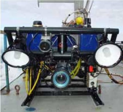
Helia, an ROV carrying a High Definition TV camera sits on the stern of the RV *Connecticut*.
