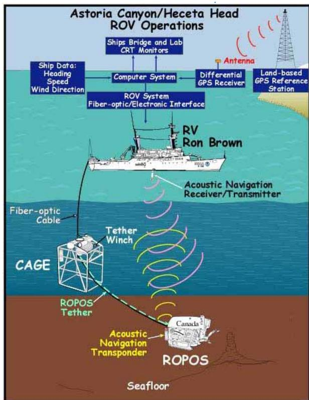
Schematic image of ROV deployment and support equipment. (Drawing is not to scale.). Image courtesy of Lewis and Clark 2001, NOAA/OER.
