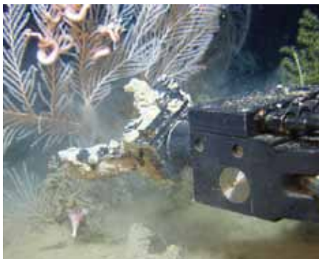
The ROV manipulator arm allows scientists to collect and bring samples to the surface for closer study. Image courtesy of Lophelia II 2008: Deepwater Coral Expedition: Reefs, Rigs, and Wrecks. http://oceanexplorer.noaa.gov/explorations/08lophelia/logs/sept29/media/falcon_rov_arm.html
