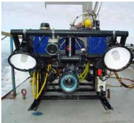
Helia, an ROV carrying a High Definition TV camera (foreground) and Isis, a towed sled with auxiliary lighting, sit on the stern of the RV Connecticut.
