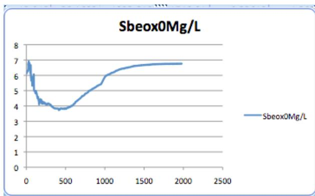
**5. Oceanographers like to plot CTD data** with depth on the y-axis and the greatest depths at the bottom of the plot, since that is the way we usually think about a profile of the water column. For an x-y plot, Excel plots the first column on the x-axis. So, to make an “oceanographer’s plot” we need to re-arrange the data so that temperature values come before depth values.
