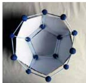
8. Repeat Step 7 four more times to form the remaining faces for the bottom half of the cage.
