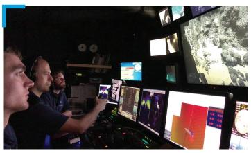
The ROV pilot controls ROV *Deep Discoverer's* grasping arm, while the co-pilot points the main camera. *Image courtesy of NOAA Ocean Exploration, American Samoa..*
