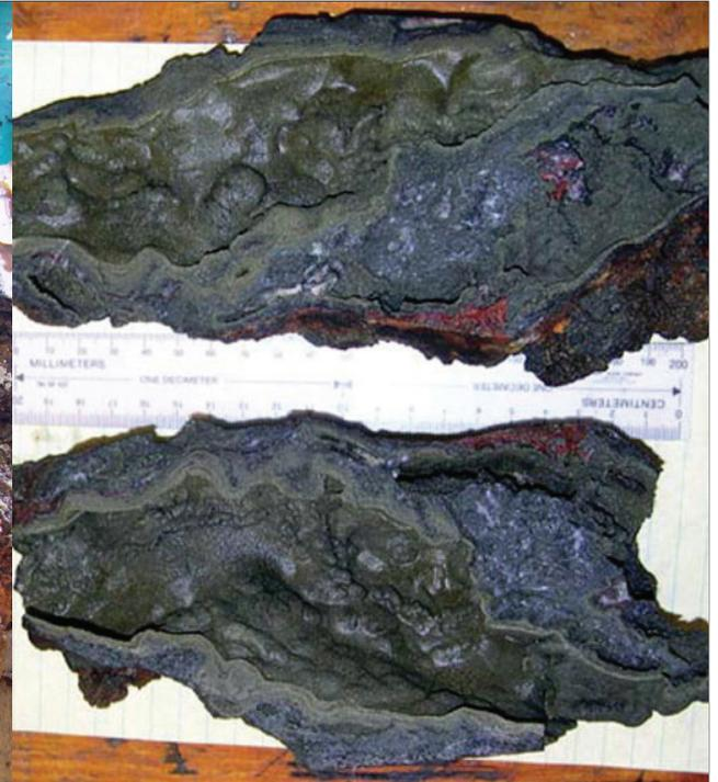
A piece of a chimney spire collected from the slope of the East Diamante volcano in the Mariana volcanic arc. It has been cut in half and is 22 cm long. The interior of the chimney is lined by a copper-rich mineral called chalcopyrite. The gray-and-white zone near the exterior of the chimney is composed of iron, zinc and barium-rich minerals called pyrite, sphalerite and barite. *Image courtesy of NOAA Vents Program.*
