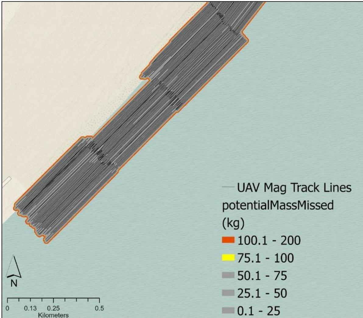
Figure 14. Example of aerial magnetometer track lines overlaid on raster surface depicting potential mass missed estimates in the WI survey area. Image: NOAA.
