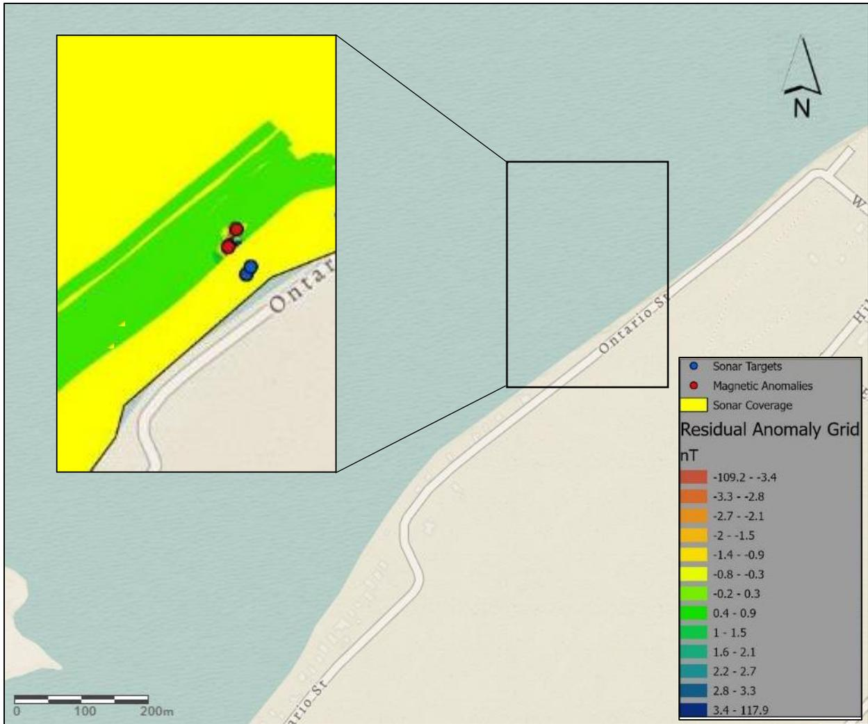
Figure 41. Detail of side-scan sonar and magnetometer data recorded around Sackets Harbor Oil Dock. Note grouping of magnetic anomalies and sonar targets. Image: NOAA.
