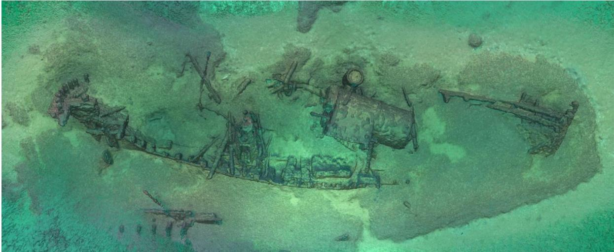
Figure 35. Photogrammetric Model of the *Henry Gust* wreck site. As the model is scaled, it can be overlaid with additional remote sensing data. Image: NOAA.
