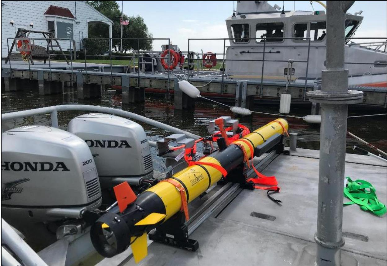
Figure 6. The University of Delaware Iver3 AUV onboard NOAA vessel R3012, ready to transit to a survey location. Image: NOAA.
