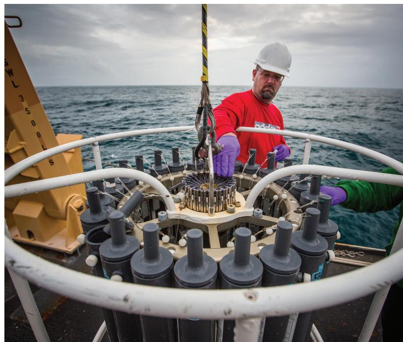
currently installed on the CTD measure altitude, light scattering (LSS), dissolved oxygen (DO), and oxygen reduction potential (ORP).
