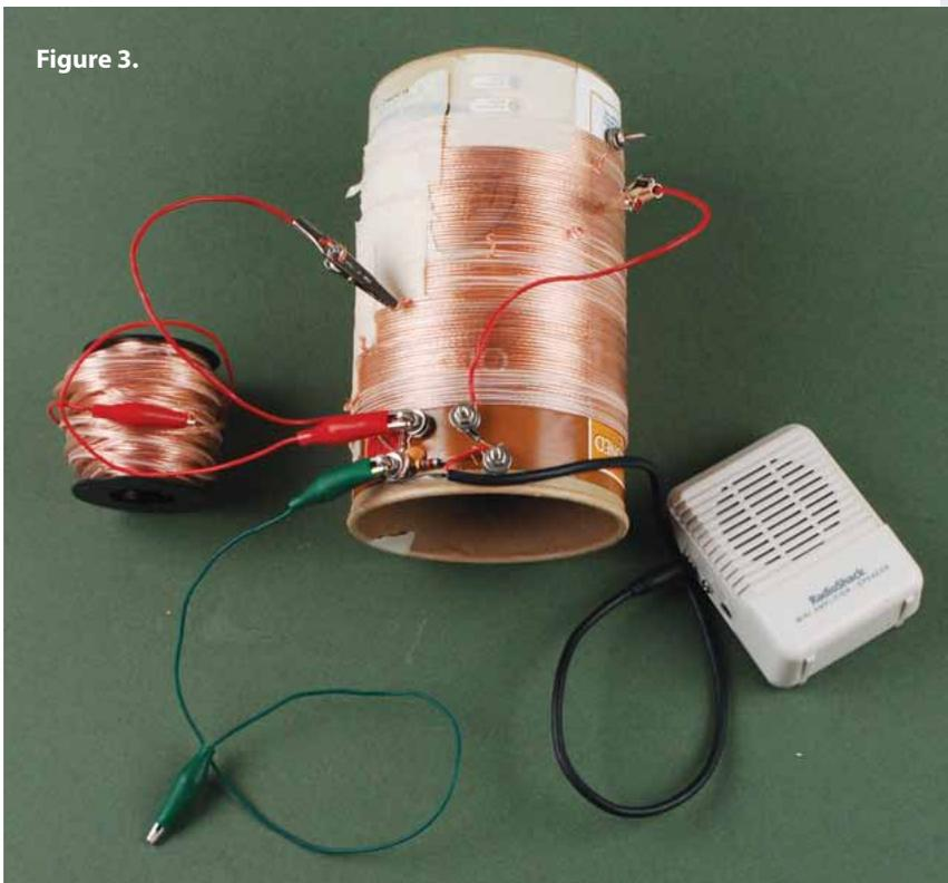
Figure 3. **A crystal radio.** Green jumper wire connects to cold water pipe (ground). Red jumper wire connects to 50-ft antenna (coiled on spool).
