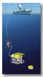
The vessel has a hull-mounted, first-of-its kind multi-beam mapping system, which will produce high resolution maps of the seafloor. The maps will be used to identify unique seafloor features for further exploration and will provide a road map for exploring a particular site with the remotely-operated vehicles (ROVs).
