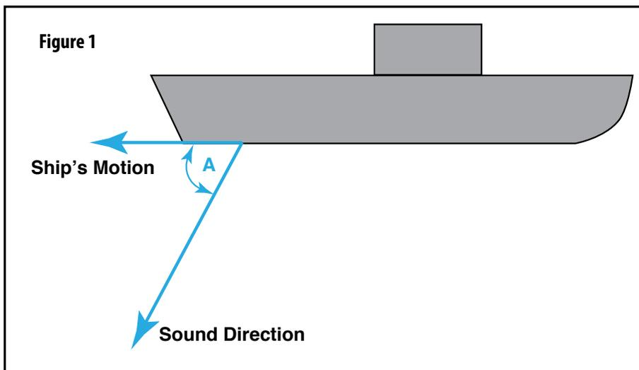
2. Our formula that relates Doppler shift to a ship's speed is  $F_d = 2 \cdot F_s \cdot (V/C)$ . But this formula will only work if surface that reflects the transmitted sound is directly ahead of the ship. Since this arrangement is not practical, the sound transmitter aboard the ship will have to point at an angle to the horizontal as shown in Figure 1. How could you modify the formula to account for the angular direction of the transmitted sound?
