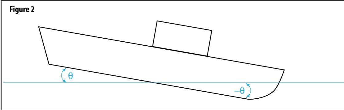
3. In heavy weather, ships tend to move up and down around an axis that passes from side to side through the middle of the ship. In other words, the bow goes up as the stern moves down, then the bow goes down as the stern moves up. This motion is called pitch or heave. This motion would change the angle shown in Figure 2, and would cause an incorrect estimate of the ship's speed. How could you compensate for this motion?
