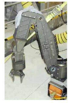
The robotic arm for the ROV Tiburon has to be both powerful and dextrous to collect many different sample types. Image courtesy of Davidson Seamount Exploration 2002, NOAA/OER. http://oceanexplorer.noaa.gov/explorations/02davidson/logs/ may20/media/fig1.html
