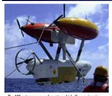
The ABE autonomous underwater vehicle (free-swimming robot). ABE (full name: Autonomous Benthic Explorer) has been used on multiple expeditions to find new hydrothermal vents in the deep ocean all over the world, from New Zealand to South Africa and from Brazil to Ecuador. Photo courtesy of Christopher German.
