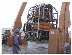
ROPOS being deployed for deep water operations inside its steel cage. http://oceanexplorer.noaa.gov/technology/ subs/ropos/media/roposfirstdive.html
