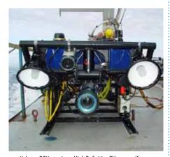
Hela, an ROV carrying a High Definition TV camera (foreground) and Isis, a towed sled with auxiliary lighting, sit on the stern of the RV Connecticut.
