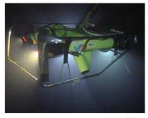
Lights and video cameras equip ROVs, enabling the operator to navigate below the ocean's surface. The S2 Phantom ROV, shown above, can move horizontally, vertically, or laterally. Image credit: NOAA.
