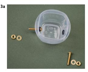
3. Starting from the inside portion of each grommet, install a stainless steel bolt through the grommet, and place a stainless steel washer and stainless steel nut onto the bolt. Hold the bolt with a screwdriver, and tighten the nut until the rubber grommet is slightly compressed. Do not crush the grommet.
