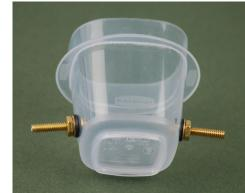
4. Pour water into the plastic container until it is about half full. Check to be sure no water is leaking around the bolt or grommet. If there is a leak, tighten the nut a little more. This assembly is called a conductivity cell.
