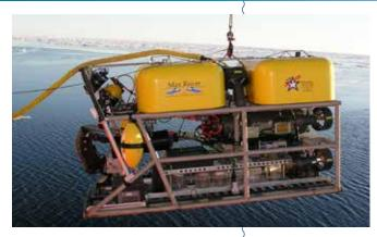
ROV Global Explorer will be used for both pelagic and benthic work. Equipped with new 4K cameras, this ROV will yield ultra-high-definition quality imaging of in situ habitats and communities, plus specimen collection capabilities essential for the discovery of delicate pelagic and benthic species. Image courtesy Deep Sea Systems. photographic equipment will be included on the Expedition's ROV *Global Explorer*.
