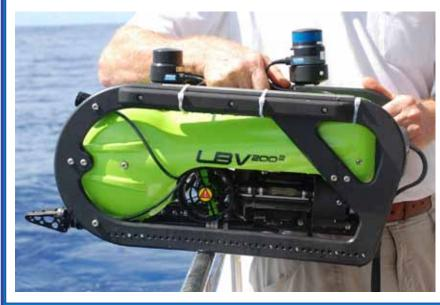
The SeaBotix LBV (little benthic vehicle) is a remotely operated vehicle (ROV) that researchers will use to explore potential underwater caves. Its small size (just 21 inches in length) makes it an ideal tool for exploring small underwater spaces. Image courtesy of Bermuda: Search for Deep Water Caves 2009 Exploration.
