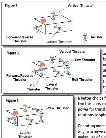
6. Have students complete Part B of the *Underwater Robot Motion Inquiry Guide*, then have each group present their results. If three thrusters are located so that the force of each thruster is directed exactly along a single axis, then these three thrusters will provide lateral, forward/reverse, and vertical motion along the x-, y-, and z-axes, respectively (Figure 2). Adding
