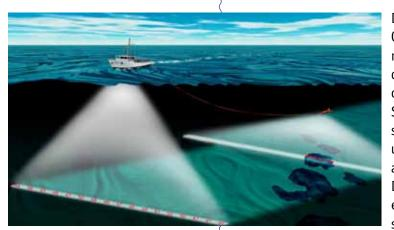
Use of multibeam sonar to map the seafloor. Image courtesy of Jill Heinerth, Bermuda: Search for Deep Water Caves 2009. http://oceanexplorer.noaa.gov/ explorations/09bermuda/background/multibeam/ media/multibeam\_fig3.html
