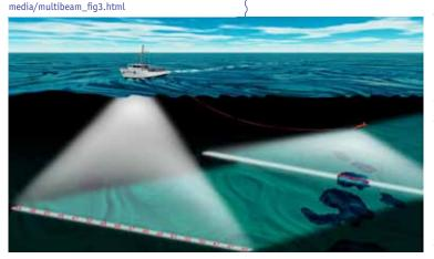
Use of multibeam sonar to map the seafloor. Image courtesy of Jill Heinerth, Bermuda:
