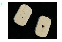
Drill two 1/16" diameter holes in one of the short wood pieces in the locations indicated on Pattern 1. Drill one 1/4" hole in the other short wood piece as indicated on the pattern.
