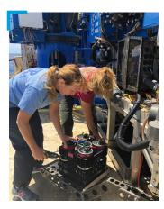
The science team removes coral quivers from the swing arm of ROV Jason. Coral quivers are containers designed to hold individual samples of coral. Image courtesy of DEEP SEARCH 2019 - BOEM, USGS, NOAA.
