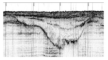
Buried paleo-river channels, flood plains, and other physical features can be detected using an acoustic instrument called a **sub-bottom profiler**. This device uses sound to penetrate sediment layers and create a two-dimensional image of the buried sediment structure that archaeologists can study to understand how humans may have interfaced with their surrounding environment.
