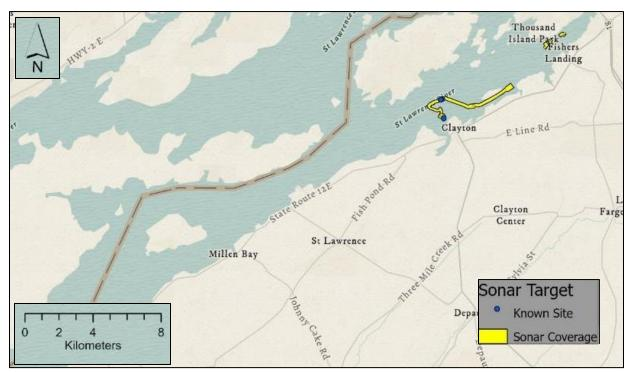
Figure 40. Polygons showing areas of side-scan sonar coverage in New York/Lake Ontario study area with picked target points overlaid. Of 34 targets, 25 were previously unidentified features and 9 corresponded with known historic vessel remains. Not all survey areas shown due to map scaling. Image: NOAA.
