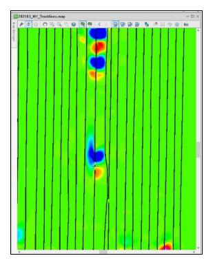
Figure 10. Example of an asymmetric dipole anomaly consisting of a slight shift in one direction followed by a substantially higher shift in the opposite direction. In the above example, a 1.5 nT positive shift is followed by a greater -24.5 nT negative shift. Like a dipole, these appear as two distinct lobes on the gridded map view with one lobe being larger and more prominent. Image: NOAA.
