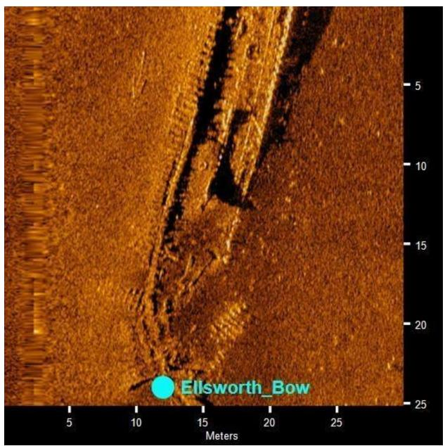
Figure 52. Side-scan sonar image of the bow of the *Ellsworth*. Image: NOAA.
