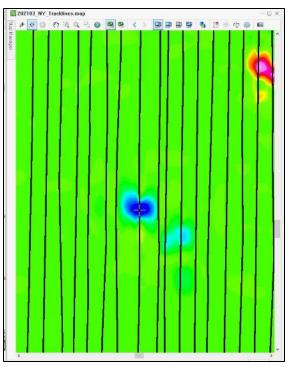
Figure 8. Example of a negative monopole presenting as a single negative shift on the map. Image: NOAA.
