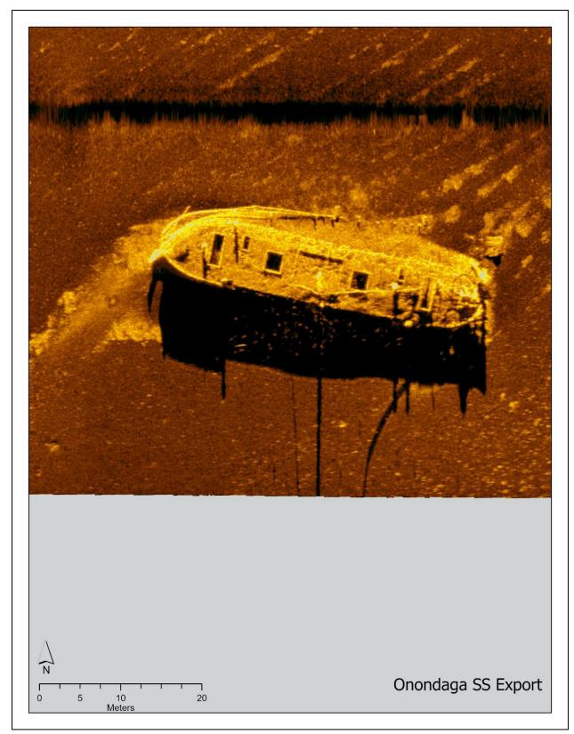
Figure 47. AUV-based side-scan sonar images collected over the site of *Onondaga's* historic vessel remains. Image: NOAA; Side-scan sonar processing: University of Delaware.
