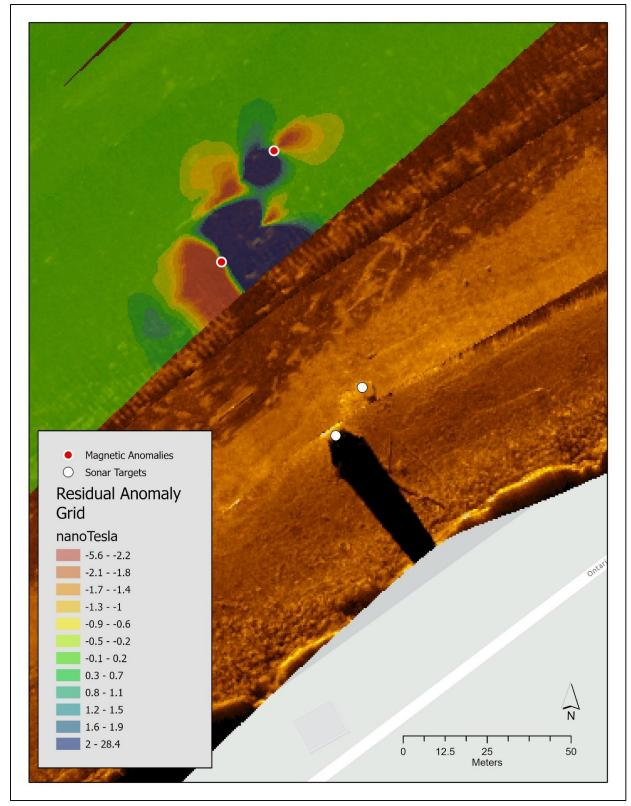
Figure 42. View of adjacent magnetometer and side-scan sonar contacts located in the vicinity of Sackets Harbor Oil Dock. Concurrent targets and anomalies are associated with the derelict oil dock structure adjacent to the Sackets Harbor Battlefield State Historic Site. Map: NOAA; Side-scan sonar processing: NOAA.
