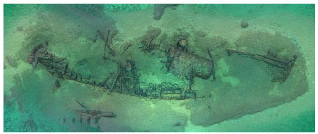
Figure 35. Photogrammetric Model of the *Henry Gust* wreck site. As the model is scaled, it can be overlaid with additional remote sensing data. Image: NOAA.
