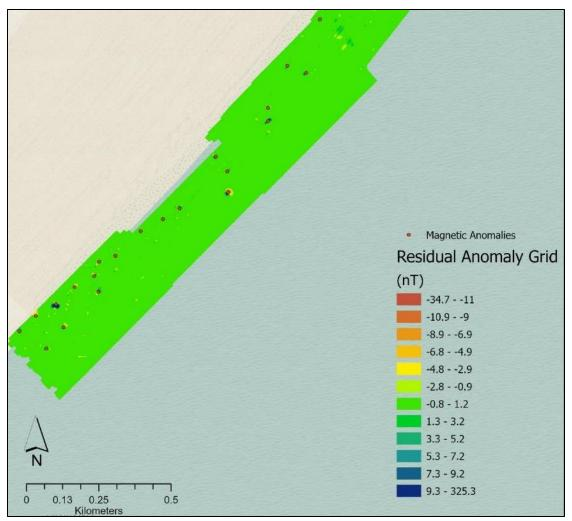
Figure 27. Detail from processed magnetic survey results within the Wisconsin/Lake Michigan study area represented as the residual anomaly grid with picked anomaly points overlaid. Image: NOAA.
