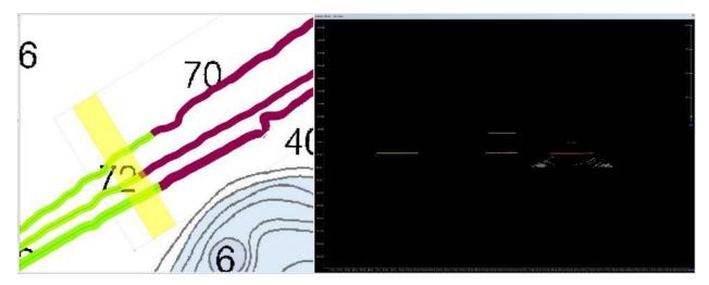
Figure 22. Nearshore area of ASV transit lines showing substantial vertical reference issues. Between port and Lime Barrell Shoals, negative depth values were registered until an abrupt switch along track to correct values. Image: NOAA.
