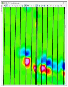
Figure 9. Example of a dipole anomaly where negative and positive shifts occur in nearly equal magnitude and appear as two distinct lobes on the gridded map view. Image: NOAA.
