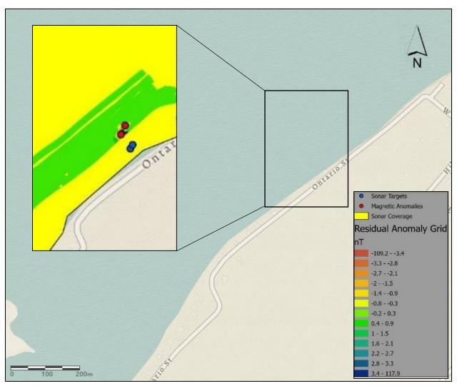
Figure 41. Detail of side-scan sonar and magnetometer data recorded around Sackets Harbor Oil Dock. Note grouping of magnetic anomalies and sonar targets. Image: NOAA.
