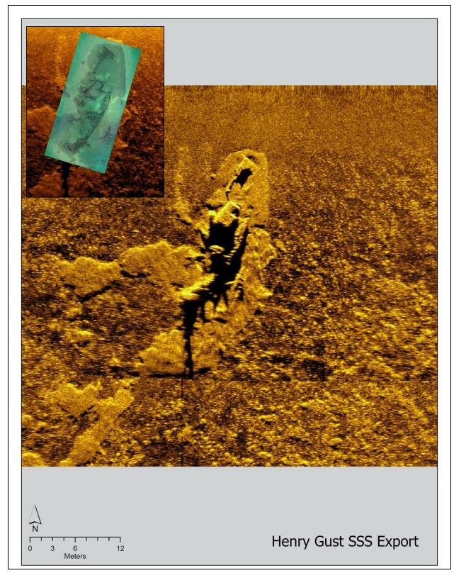
Figure 30. AUV-based side-scan sonar images collected over the site of *Henry Gust's* historic vessel remains. Top left inset shows a photogrammetric model overlaid with the shipwreck site (no scale). Map: NOAA; Side-scan sonar processing: University of Delaware.
