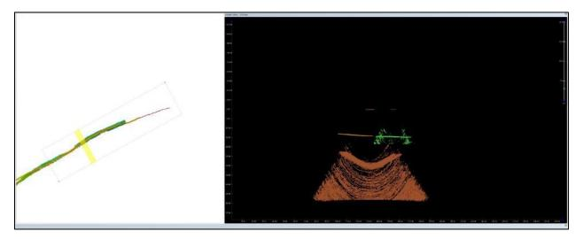
Figure 20. View of CARIS Subset Editor showing across track line fliers due to sensor noise. Image: NOAA.
