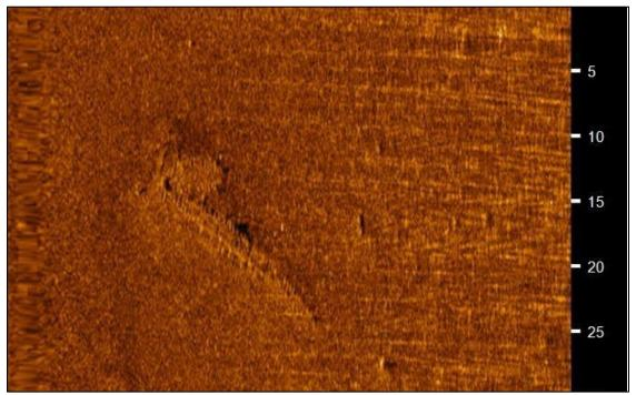
Figure 48. Side-scan sonar image of Survey Area 3\_10. Note oblong shape consisting of potential frames, presumably attached to a keel timber. Scale bar is in meters. Image: NOAA.
