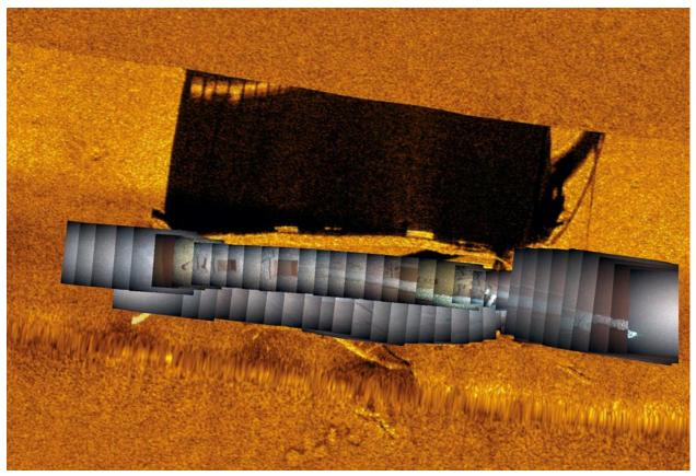
Figure 32. *Gallinipper* AUV based side-scan sonar mosaic with AUV photo overlay. Overlapping AUV photos were also stitched into seamless image mosaics using Agisoft Metashape photogrammetric software. Image: University of Delaware.
