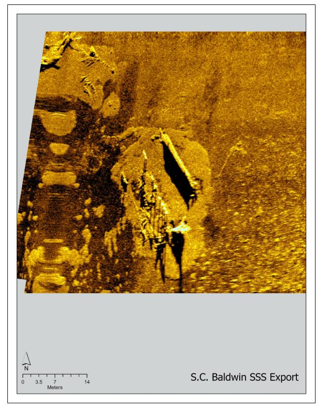
Figure 29. AUV-based side-scan sonar images collected over the site of *S.C. Baldwin's* historic vessel remains. Map: NOAA; Side-scan sonar processing: University of Delaware.
