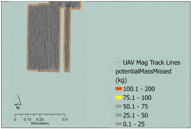
Figure 15. Detail of aerial magnetometer track lines overlaid on raster surfaces depicting potential mass missed estimates in the NY survey area. Image: NOAA.
