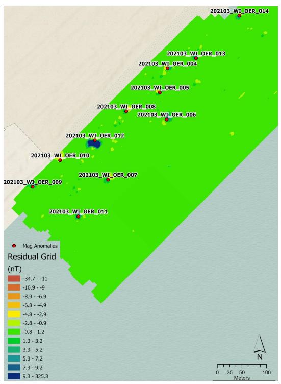
Figure 34. Detail of several magnetometer anomalies within the Wisconsin/Lake Michigan study area. Individual anomalies represented as the residual anomaly grid with picked anomaly points overlaid. Image: NOAA.
