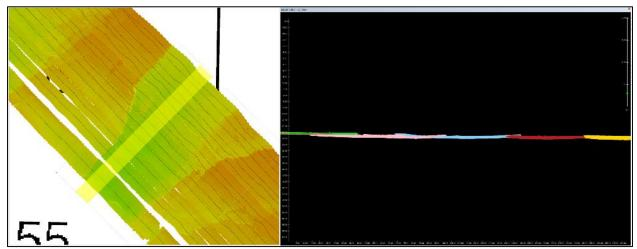
Figure 44. Plan view (left) and cross section view (right) of processed MBES data exhibiting sound velocity errors and motion artifacts in data files causing misalignment. Image: NOAA.
