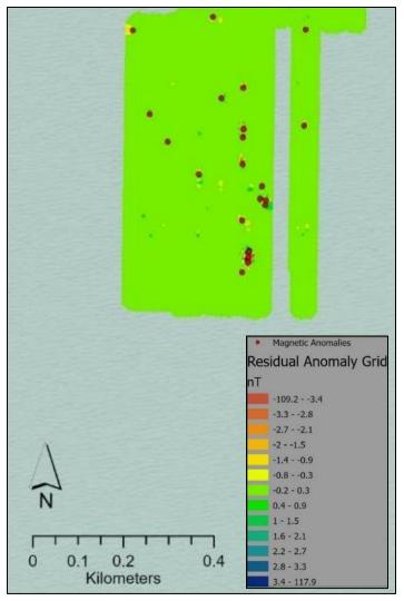
Figure 39. Detail of processed magnetic survey results within the New York/Lake Ontario study area represented as the residual anomaly grid with picked anomaly points overlaid. Image: NOAA.
