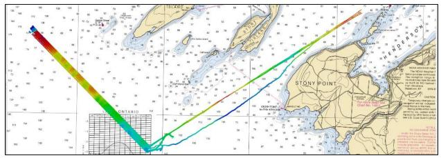
Figure 43. Processed MBES bathymetry gridded at 1 m within the New York/Lake Ontario study area. Image: NOAA.
