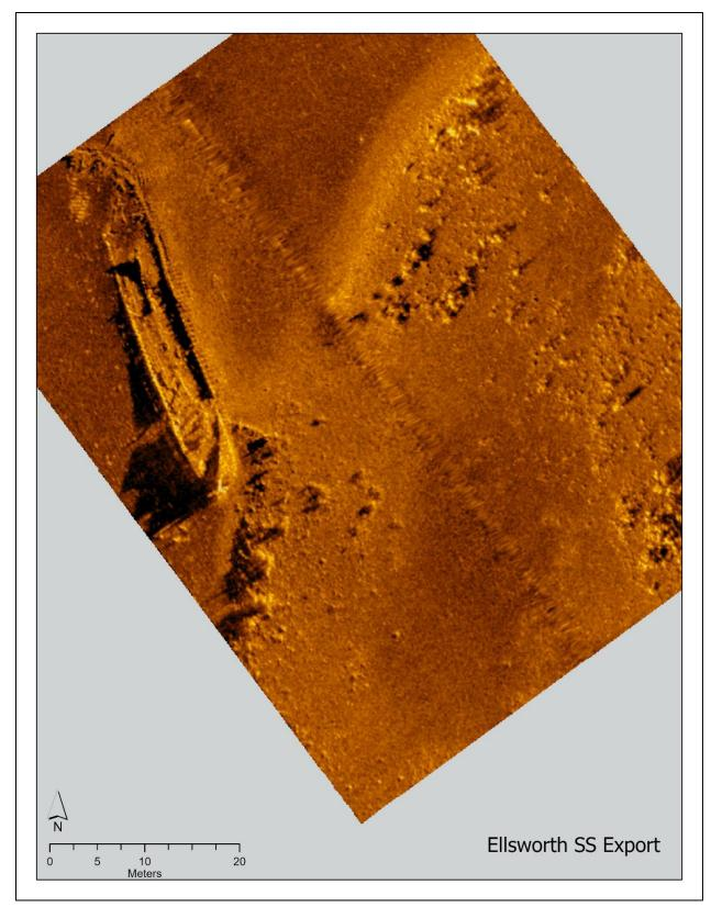
Figure 46. AUV-based side-scan sonar images collected over the site of *Ellsworth's* historic vessel remains. Image: NOAA; Side-scan sonar processing: NOAA.
