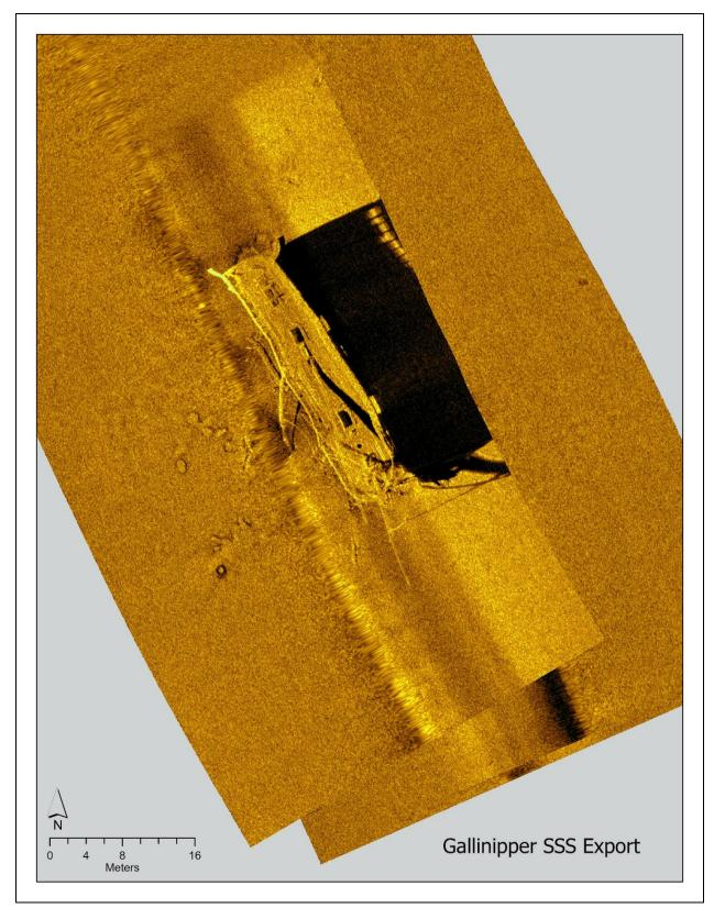
Figure 31. AUV-based side-scan sonar images collected over the site of *Gallinipper's* historic vessel remains. Map: NOAA; Side-scan sonar processing: University of Delaware.
