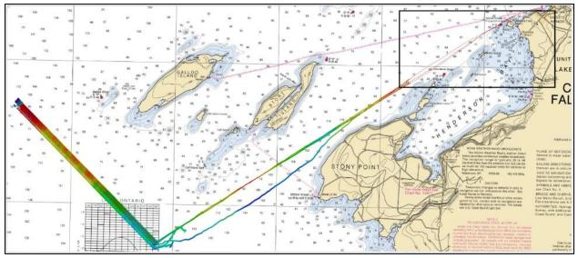
Figure 21. Processed MBES data within the NY project area. Accepted survey lines included 3 transit lines and 14 run lines within the offshore survey block. Image: NOAA.
