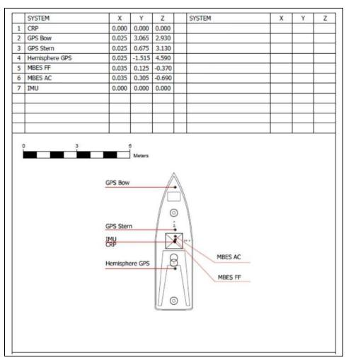
Figure 16. Instrument offsets for the C-Worker 8 ASV operated by Ocean Infinity to conduct MBES operations in Lake Michigan and Lake Huron. Image: Ocean Infinity.
