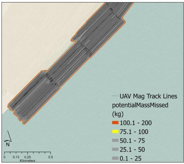
Figure 14. Example of aerial magnetometer track lines overlaid on raster surface depicting potential mass missed estimates in the WI survey area. Image: NOAA.
