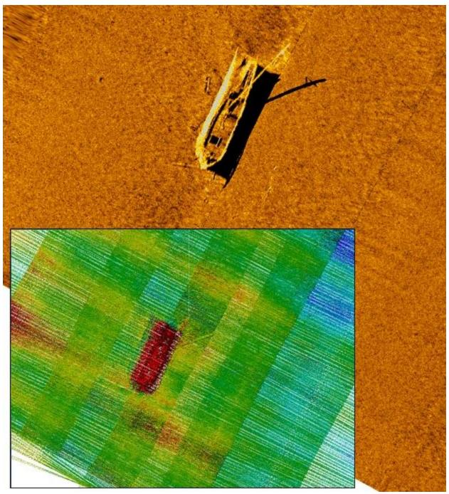
Figure 33. Side-scan sonar acoustic image of the shipwreck *Home*. Bathymetric acoustic imagery of *Home* collected via the Iver3 AUV can be seen in the bottom left. Side-scan sonar and multibeam sonar processing: University of Delaware.
