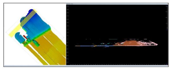
Figure 19. View of CARIS Subset Editor showing cross section point cloud of turn data in the C-Worker 8 ASV files. Sonar data logged during turns required substantial cleaning to remove erroneous soundings. Image: NOAA.
