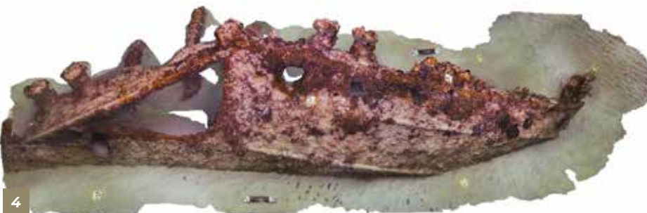
4. Perspective view of the shipwreck's stern created from hundreds of still images meshed together through computer processing (NOAA and UM-RSMAS).
