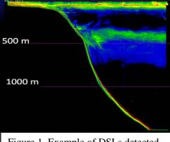
Figure 1. Example of DSLs detected at 38 kHz interacting with the continental shelf/slope at night in the Gulf of Mexico (Boswell unpub.
