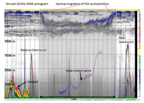
Figure 1. 18-kHz echogram along a transect from Balanus to Bear Seamounts on 28-29 July 2016. The seabed echo is the rainbow color feature near the bottom of the echogram and a false (aka "ghost") echo is highlighted in purple. The acoustic scattering from about 400 to 1000 m is the DSL.
