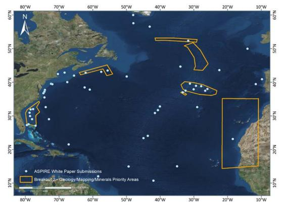
**Figure 12.** Map showing geology, mapping, and minerals geographic priority areas identified during breakout session 2. White dots are the general location of white paper submissions; orange polygons are priority areas for exploration identified during the workshop discussions.
