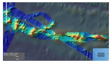
Figure 2: Existing multibeam bathymetry for seamounts of Research Ridge from a 2014 cruise on the R/V Knorr. Coverage is sparse from the central portion of the ridge and above several seamount summits.
