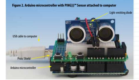
When using a particular sensor/microcontroller system for the first time, it is always a good idea to check the accuracy of the system by obtaining several measurements of an object at known distances, and comparing the measurements with the actual distances. Graphing the results of several tests can give you a good idea about the accuracy and limits of your system.
