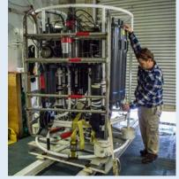
Water samples are collected from the Niskin bottles on a Conductivity, Temperature and Depth profiler (CTD). All 20 Niskin bottles take water samples from various depths, starting near the seafloor and ending close to the surface. Photo courtesy of Caitlin Bailey, GFOE, The Hidden Ocean 2016: Chukchi Borderlands. http://oceanexplorer.noaa.gov/explorations/16arctic/ logs/july/24/media/shipton.html
