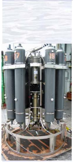
A closeup of a CTD, the primary tool used to map hydrothermal plumes. A ring of plastic sampling bottles surrounds the CTD, which is housed in the steel container in the center of the rosette. CTD sensors are visible at the bottom of the pressure case. Image courtesy of NOAA Vents Program.
