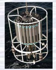
A CTD rosette with water sampling bottles attached is lowered to measure the salinity, temperature, depth and concentration of particles in the water column. Image courtesy of NOAA *Okeanos Explorer* Program, INDEX-SATAL 2010.
