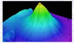
Okeanos Explorer's EM302 multibeam sonar mapping system produced this detailed image of the Kawio Barat seamount, which rises around 3800 meters from the seafloor. Image courtesy of NOAA Okeanos Explorer Program, INDEX-SATAL 2010. http://oceanexplorer.noaa.gov/okeanos/explorations/10index/ logs/hires/june26fig1\_hires.jpg
