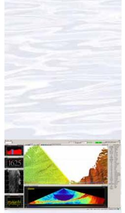
This is a screen grab from the multibeam acquisition computer during a typical mapping watch. The center area shows the coverage, on the left is the sonar signal strength, depth, backscatter and ship motion data. The bottom window is the water column display, where the sonar can also detect features such as plumes. Image courtesy of NOAA Okeanos Explorer Program, INDEX-SATAL 2010. http://oceanexplorer.noaa.gov/okeanos/explorations/10index/logs/ hires/multibeam\_acq\_hires.jpg
