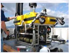
The Little Hercules remotely-operated vehicle (ROV) is a dual-body system capable of operating to depths of 4,000m. It is deployed from the Okeanos Explorer and attached to it by a tether. One vehicle is suspended above the other and serves to illuminate and image the surroundings. Image courtesy of NOAA Office of Ocean Exploration and Research.
