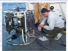
A CTD is attached to a metal frame called a rosette, or carousel along with numerous water sampling bottles. This "hydrocast" is deployed off the side of a vessel, and provides information about the composition of the water column.
