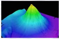
Okeanos Explorer's EM302 multibeam sonar mapping system produced this detailed image of the Kawio Barat seamount, which rises around 3800 meters from the seafloor. Image courtesy of NOAA Okeanos Explorer Program, INDEX-SATAL 2010 http://oceanexplorer.noaa.gov/okeanos/explorations/10index/
