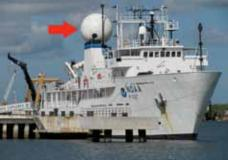
All communications with the shore are made possible by the *Okeanos Explorer*'s powerful satellite dome, which enables the ship to establish high-bandwidth connectivity with Exploration Command Centers throughout the world. Image courtesy of NOAA *Okeanos Explorer* Program, INDEX-SATAL 2010
