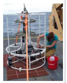
Senior Survey Technician Elaine Stuart works on the CTD while the altimeter battery recharges. Water sampling bottles, which are often attached to the rosette frame, have been removed for tow-yo operations. Sensors are mounted in the lower part of the frame where SST Stuart is working. Image courtesy of NOAA Okeanos Explorer Program.
